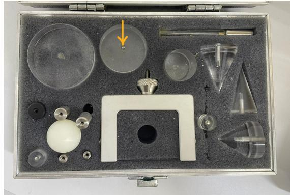
Figura 21: Cabezal TA4/1000
