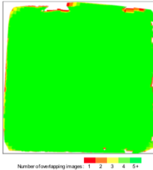
Figure 4: Number of overlapping images computed for each pixel of the orthomosaic. Red and yellow areas indicate low overlap for which poor results may be generated. Green areas indicate an overlap of over 5 images for every pixel. Good quality results will be generated as long as the number of keypoint matches is also sufficient for these areas (see Figure 5 for keypoint matches).
