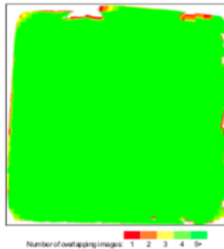
Figure 4: Number of overlapping images computed for each pixel of the orthoreosaic. Red and yellow areas indicate low overlap for which poor results may be generated. Green areas indicate an overlap of over 5 images for every pixel. Good quality results will be generated as long as the number of keypoint matches is also sufficient for these areas (see Figure 5 for keypoint matches).
