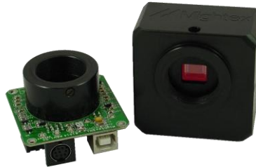
Figura 79 USB2.0 Monochrome 5MP CMOS Camera.
