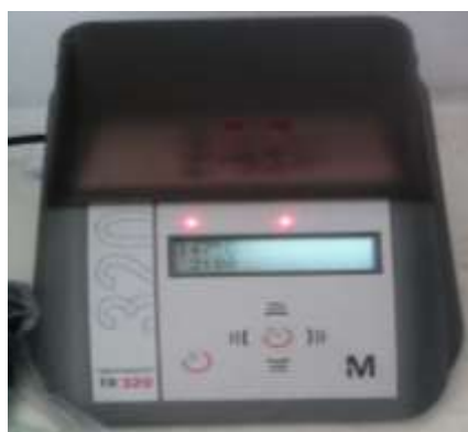
Figura No. 23 Termoreactor
