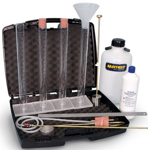
Figura 24: Equivalente de arena (MATEST, 2018)
