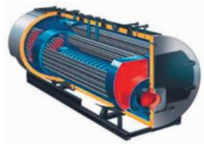
Figura 12: Detalle caldera Pirotubular
