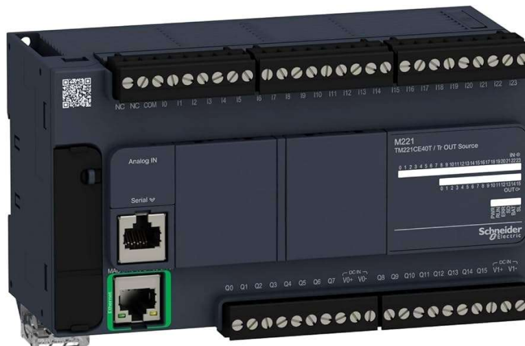
Figura 11. PLC Modicon TM221CE40T de Schneider Electric [15].
