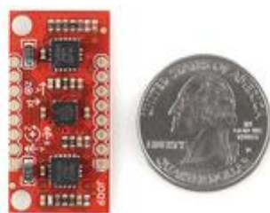
FIGURA NO. 43. IMU 6DOF [40]
