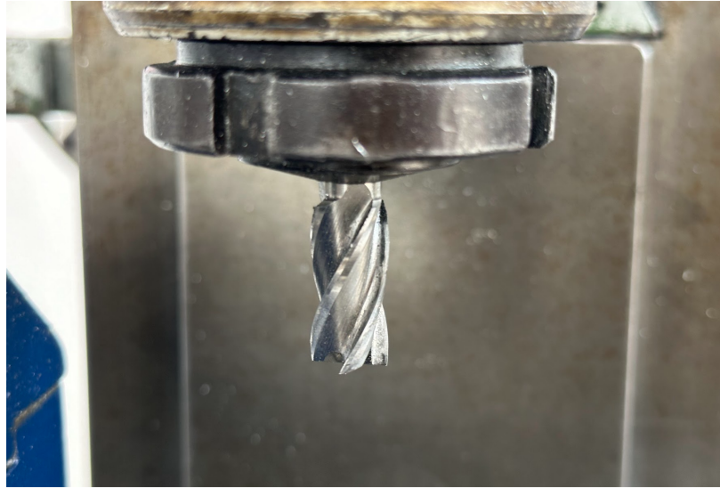
Figura 20: Fresa HSS 12 mm
