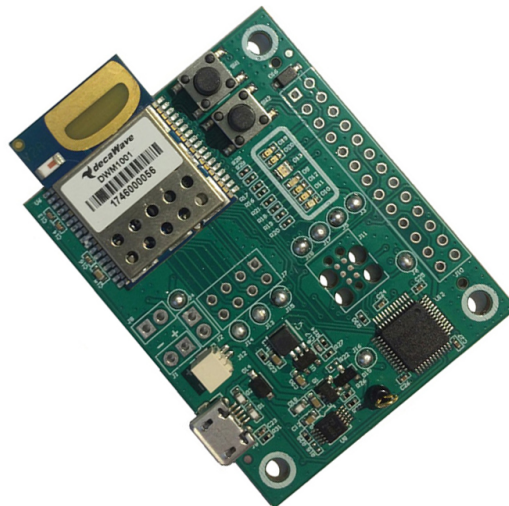
Figura 10: DWM1001 Development Board de la empresa Decawave [10]
