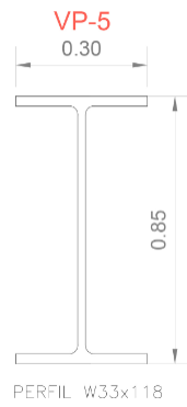
Figura 19: Viga principal VP5
