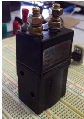
Figura 57: Contactor DC Curtis SW60-6
