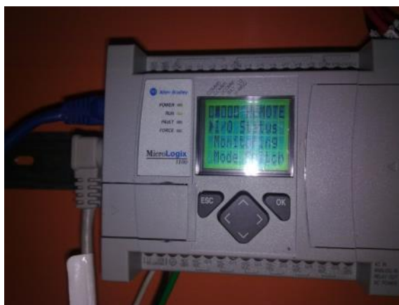
Figura 99: PLC Micrologix 1100 1763-L16AWA
