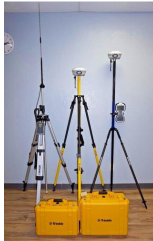
Figura 9: Base y Rover Trimble R4.
