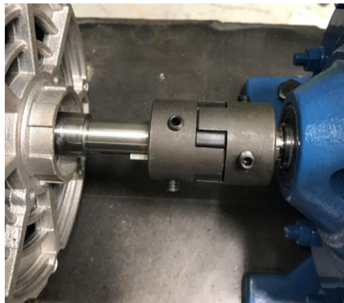
Figura No.2. Acople motor - reductor.
