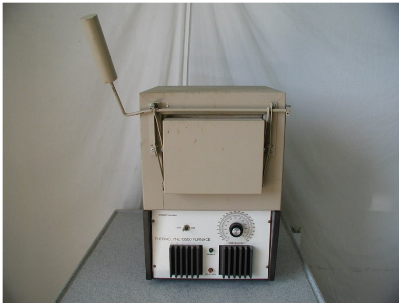
Figura No. 1: Mufla Thermolyne Model FA10525P-1, No. Serial 32501661, 120 V, 14.0 amp, 1680 Watts.
