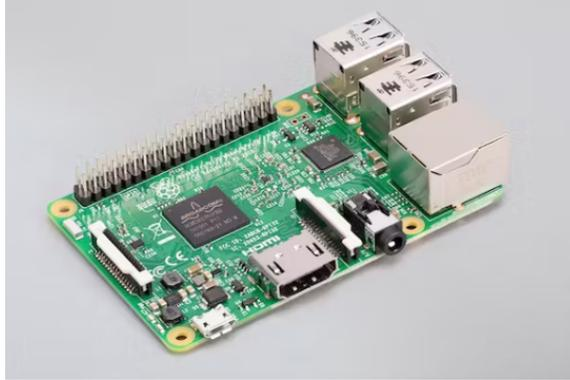
Figura 5: Raspberry Pi 3 Model B
