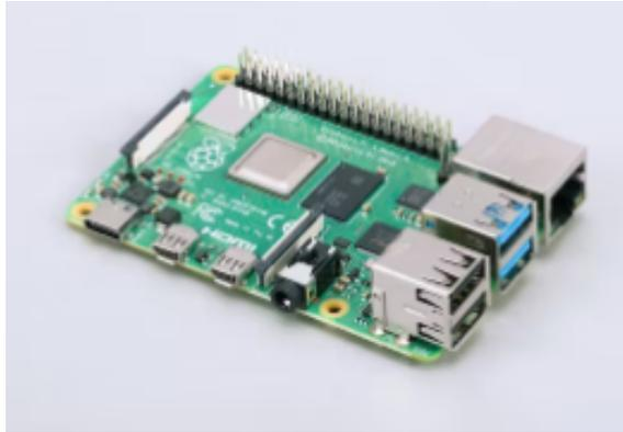
Figura 8: Raspberry Pi 4 Model B
