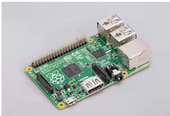
Figura 4: Raspberry Pi 1 Model B+
