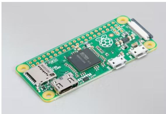
Figura 1: Raspberry Pi Zero
