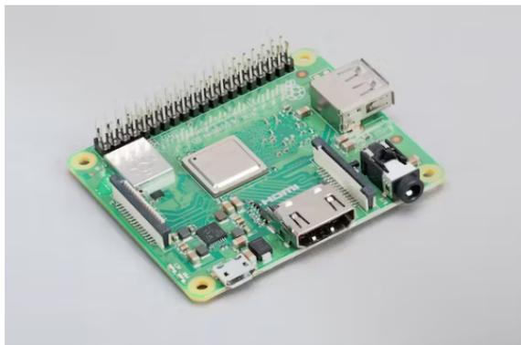
Figura 7: Raspberry Pi 3 Model A+
