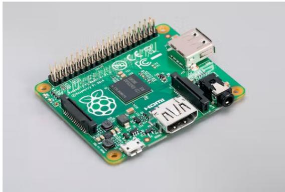
Figura 3: Raspberry Pi 1 Model A+
