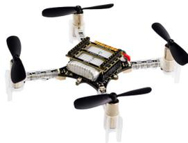
Figura 2: Quadcopter open source Crazyflie 2.0.
