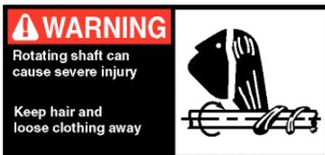
PLACED ON LINE SHAFT SIDE.
